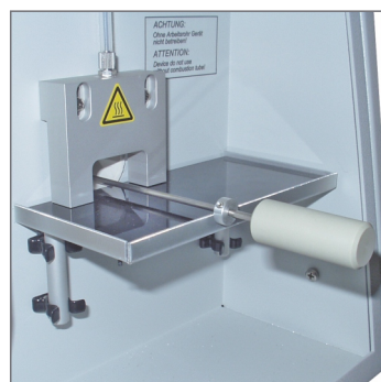
Sample dosing with boats of ceramic or quartz glass
