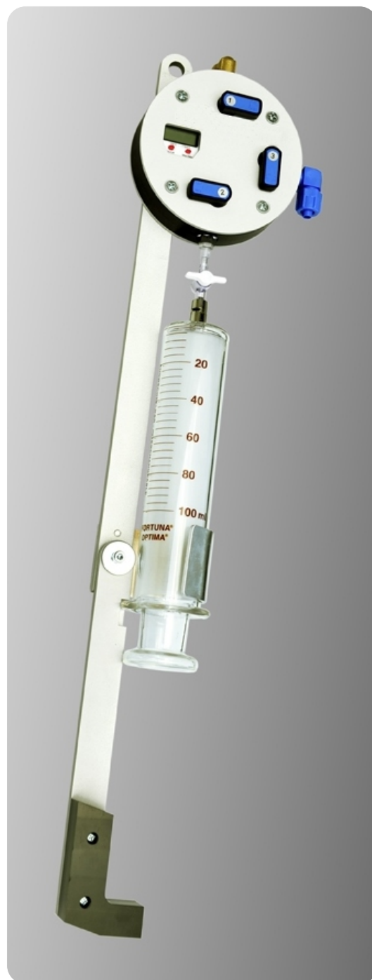
Manual Oil Sampling Kit with glass syringe (100 mL)
